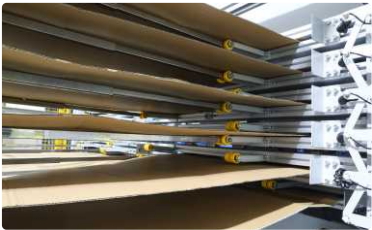
独特的防卡纸调库系统 Unique anti-jam paper transfer system
